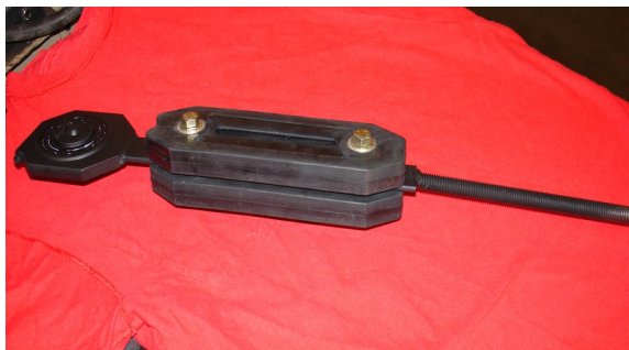
Main Shaft Clutch Assembly Eliminates Vibration
