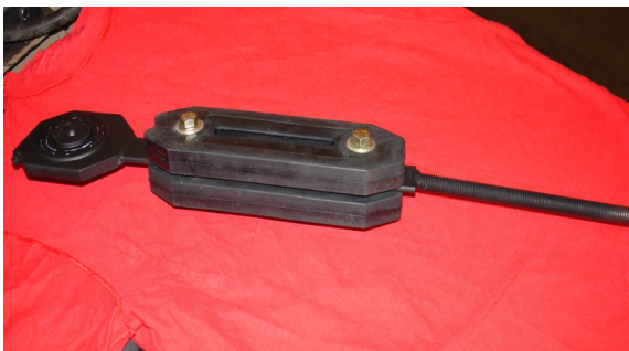
Main Shaft Clutch Assembly Eliminates Vibration
