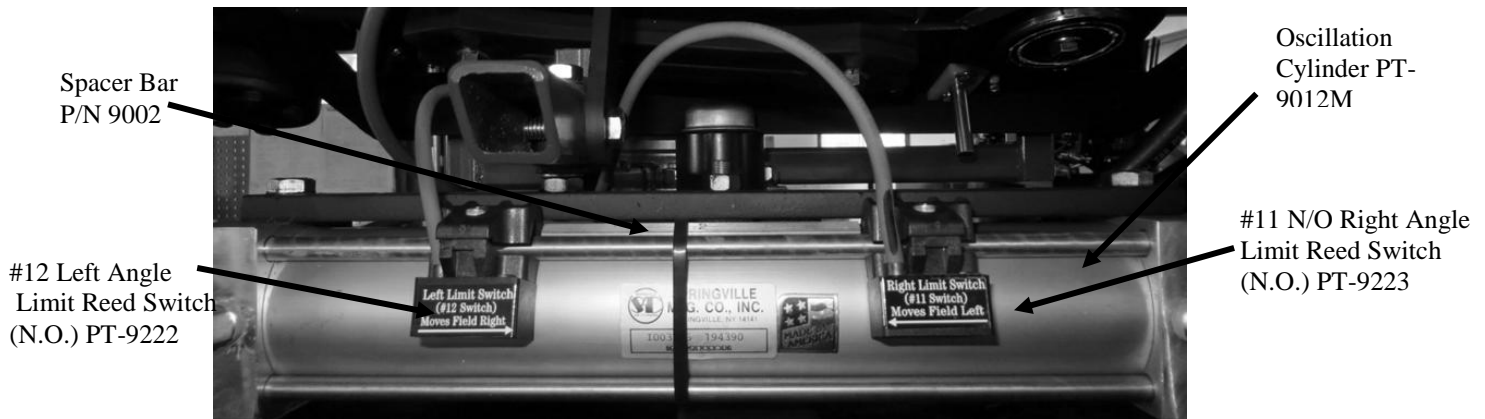
Pat-Trap® #12 & #11 Limit Reed Switches on Oscillation Cylinder
