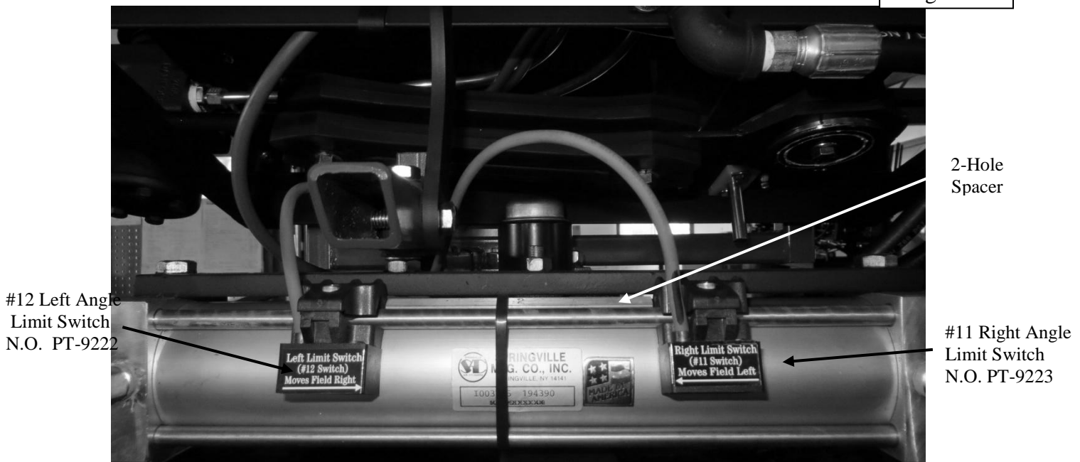
PAT-TRAP® Oscillation Cylinder with Field Angle Switches and 2-Hole Spacer Bar
